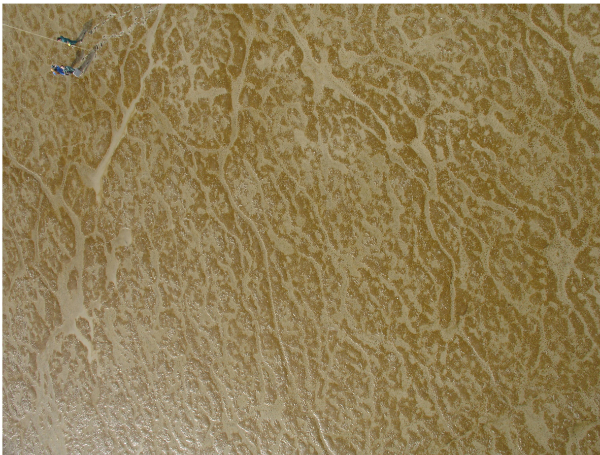
Figure B1: Aerial photograph taken for regularity analysis. Brown areas correspond to high diatom biomass, and gray areas correspond to almost bare sediment.
